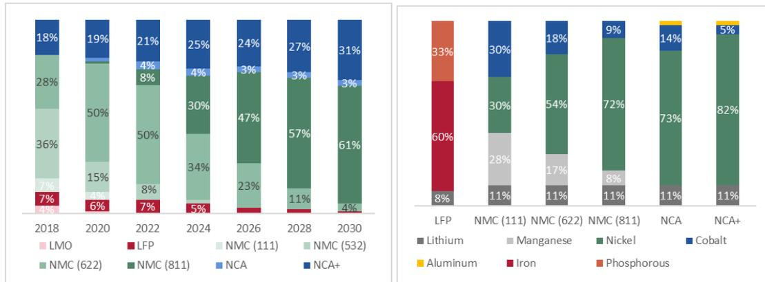
Figure 25 LHS: Evolution of Cathode chemistry on passenger EVs; RHS: Metal content of cathode chemistries<sup>52</sup>
