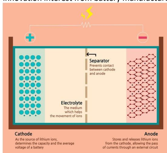
*Figure 24 Components of a Li-ion Battery*<sup>51</sup>
