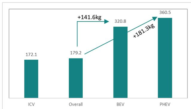
Figure 22 Average Aluminium Content per vehicle - Comparison by Powertrain Variant (Net weight in kg)<sup>46</sup>
